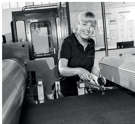
Measuring the thickness of graphite felt for the thermal insulation of high temperature furnaces
